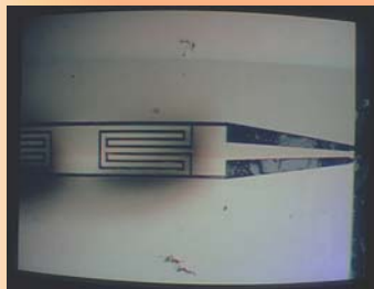
Detail of the 38GHz 4-cell opposed open-end series stub CPW filter structure supported on a 2.2 \mu\text{m} GaAs/AlGaAs membrane
