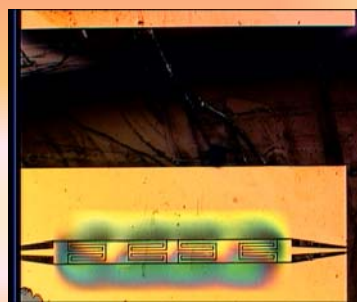
GaAs membrane supported double folded open end series stub band pass filter structure for 38 GHz
